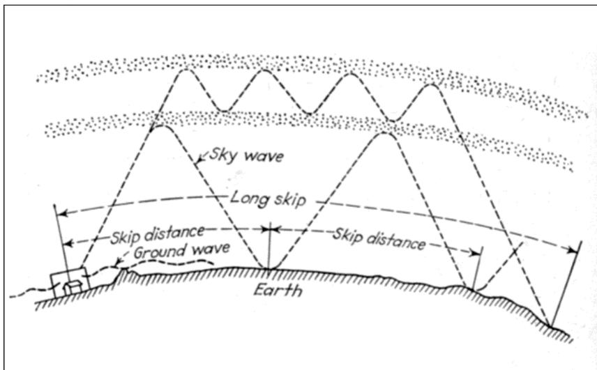
Figure 5. Charged particles in the ionosphere can reflect radio signals, which can then come back to earth quite some distance away from the transmitter.. These reflected signals often shows up at the frequencies used in the AM broadcast band, especially at night, but NOT at the much higher frequencies used for FM.
