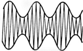
Figure 3. An amplitude modulated radio signal.
